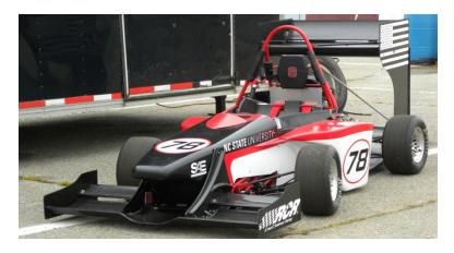
WMF-16 switched from the turbo package used since 2005 to a naturally aspirated engine. The team also returned to a pull rod suspension in the front.
