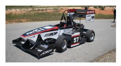
2017 was the first year that the team went to two FSAE competitions. The car featured carbon fiber suspension components and added down force. The car was the lightest in recent years at 452 lbs.
